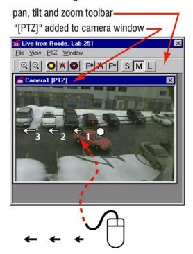
**Fig. 23.** Using the mouse to control PTZ cameras. As you move the mouse-pointer through a *PTZ camera window*, the pointer changes to a white octagon or to an arrow with a number.
